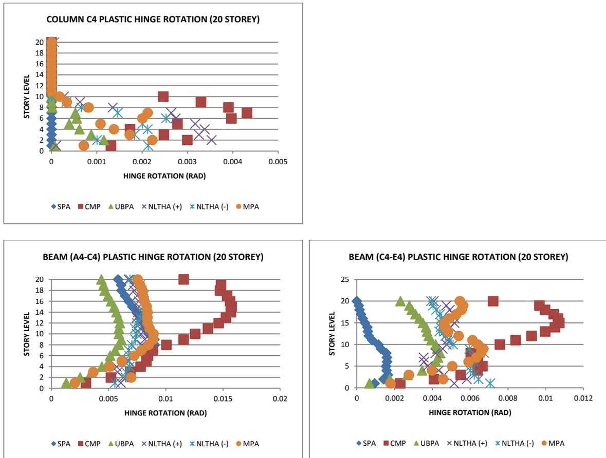
Figure 7 : Beam and column plastic hinge rotation
