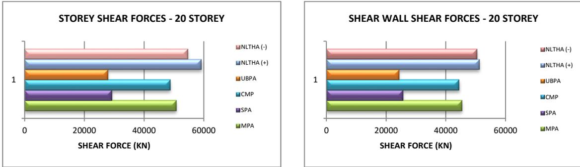
Figure 9 : Story Shear and Shear Wall Shear Force
