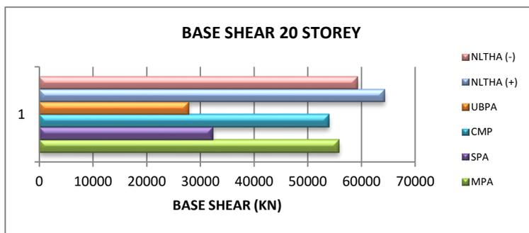
Figure 8 : Total Base Shear of 20- and 50-storey Building
