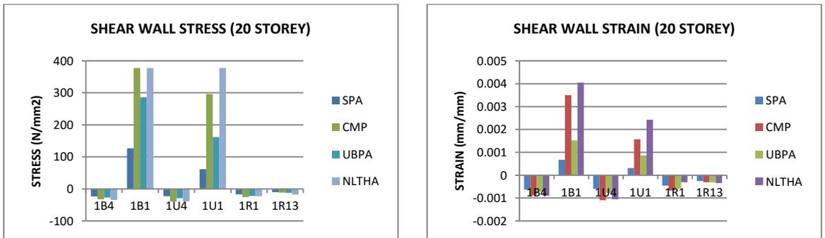
Figure 11 : Shear Wall Stress and Strain
