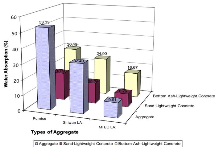
Figure 2. Water Absorption of LA, Sand-LWC and Bottom Ash- LWC
