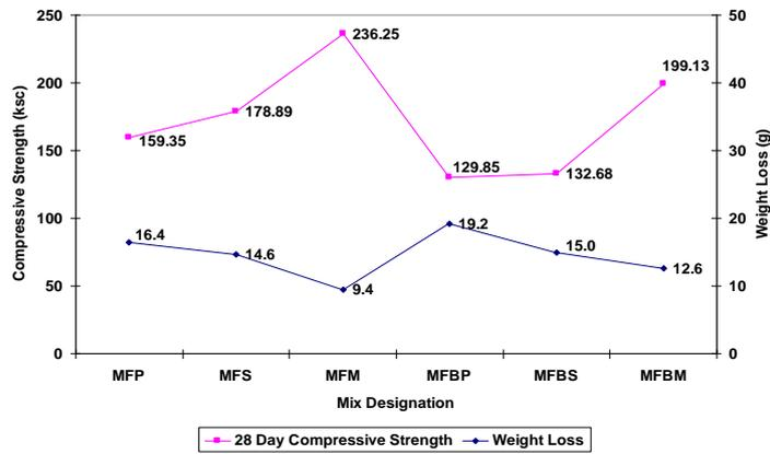
Figure 1. Relationship between Compressive Strength and Weight Loss
