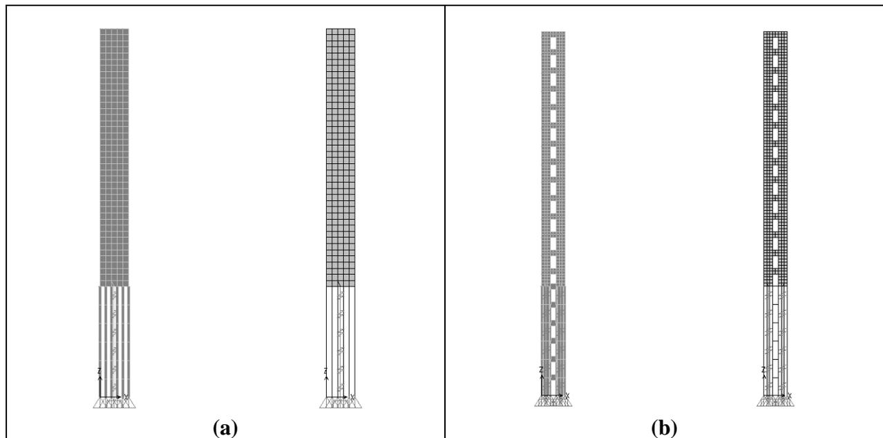
**Figure 3. (a) Fiber or frame model of plain wall; (b) Fiber or frame model of core wall with opening**
