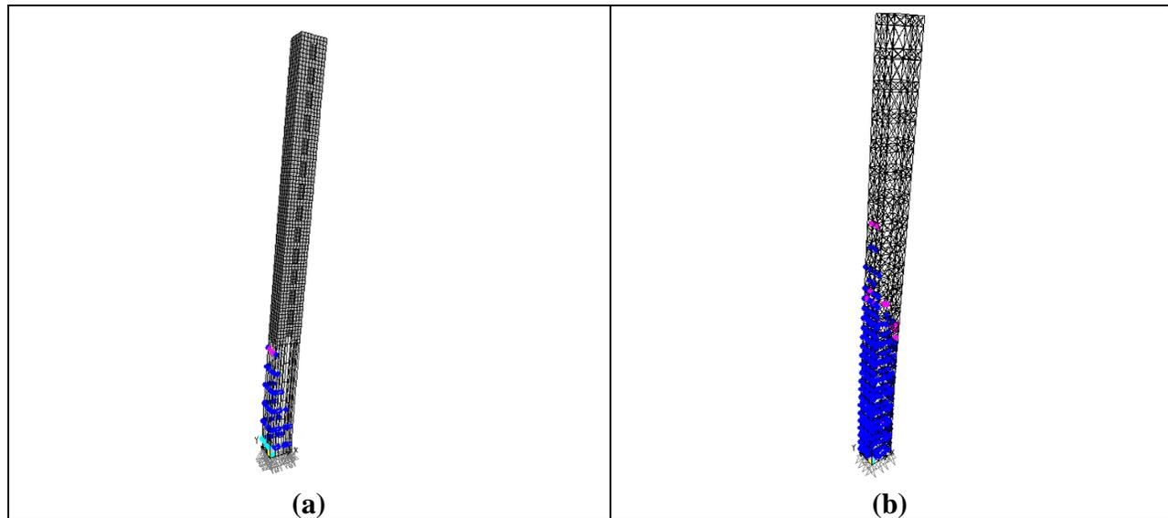
**Figure 15. (a) Hinge formation in core wall (Fiber or frame model); (b) Hinge formation in core wall (Strut and tie model)**
