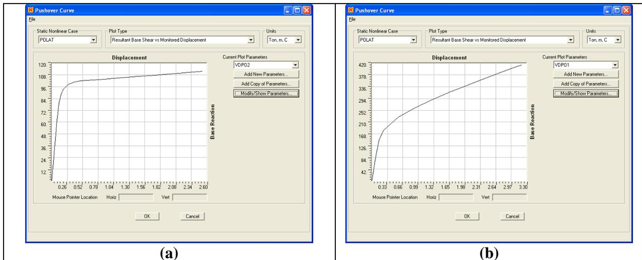
**Figure 14. (a) Base shear and top displacement of core wall (Fiber or frame model); (b) Base shear and top displacement of core wall (Strut and tie model) Unit: Ton-m**
