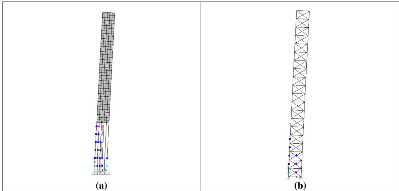
**Figure 10. (a) Hinge formation in planner wall (Fiber or frame model); (b) Hinge formation in planner wall (Strut and tie model)**
