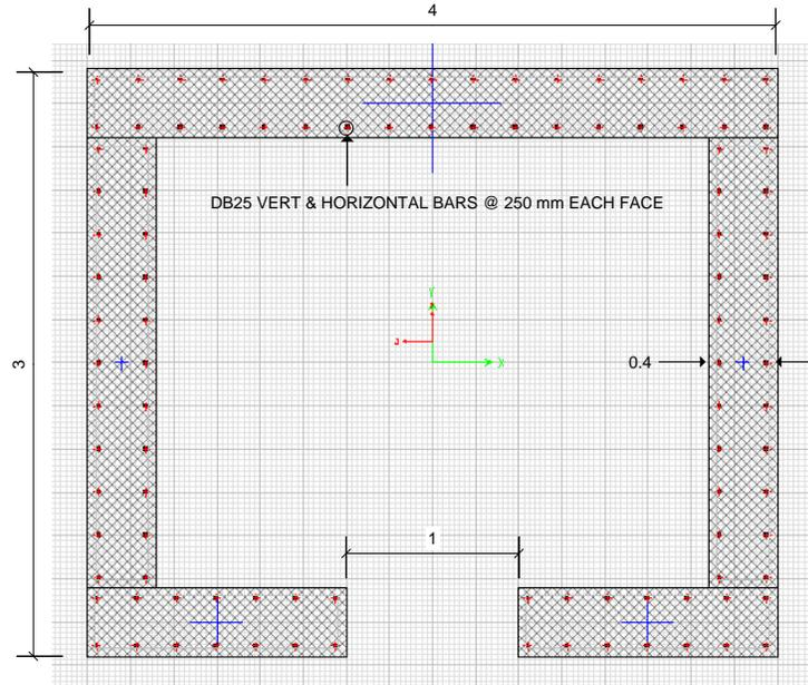
For Link Beam above opening, Top Rebar = 8-DB25, Bottom Rebar = 8-DB25
