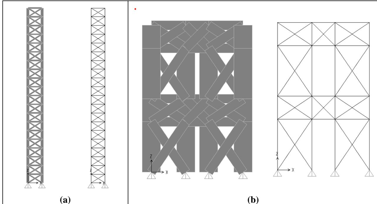
**Figure 4. (a) Strut and tie model of planner wall; (b) Strut and tie model of core wall with opening**
