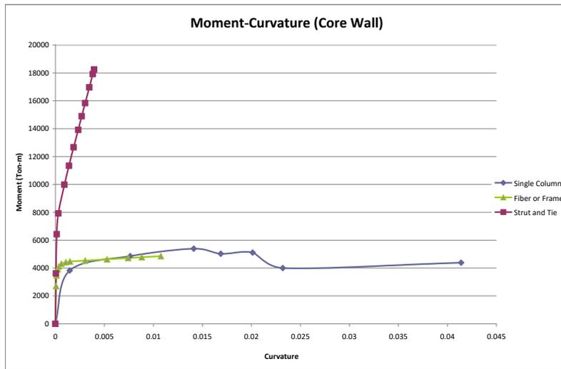
**Figure 13. Comparison of moment-curvature curves in core wall**
