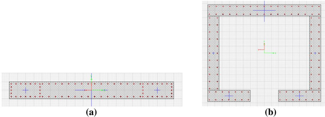
**Figure 2. (a) Frame section of planner wall; (b) Frame section of core wall with opening (link beam above the opening is not considered)**
