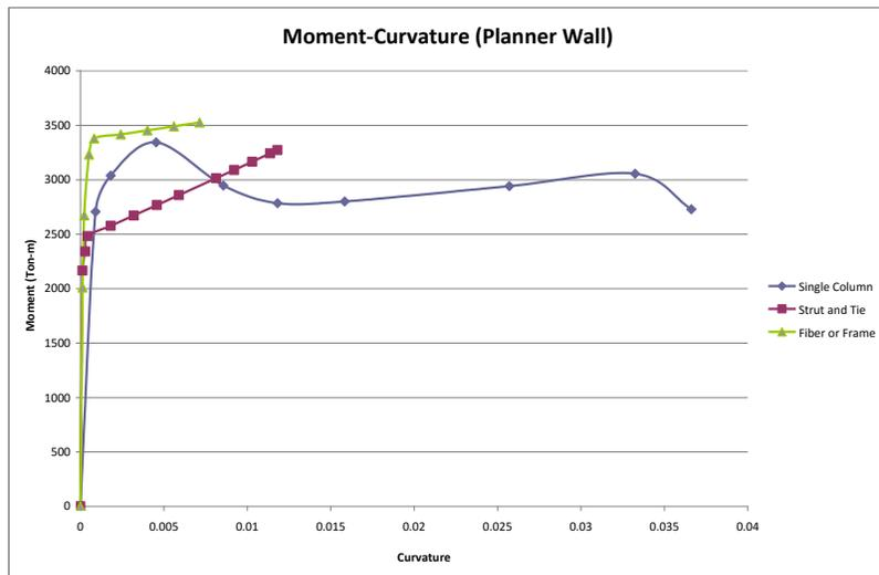
**Figure 8. Comparison of moment-curvature curves in planner wall**
