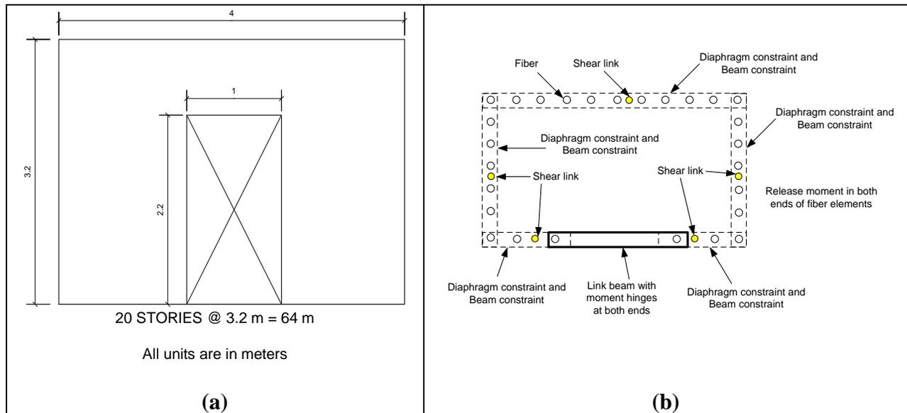
**Figure 12. (a) Elevation of opening in core wall; (b) Fiber or frame modeling in core wall**
