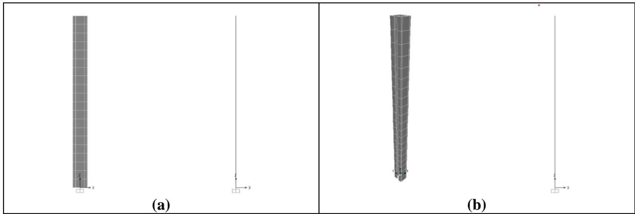
**Figure 1. (a) Single column model of planner wall; (b) Single column model of core wall with opening**
