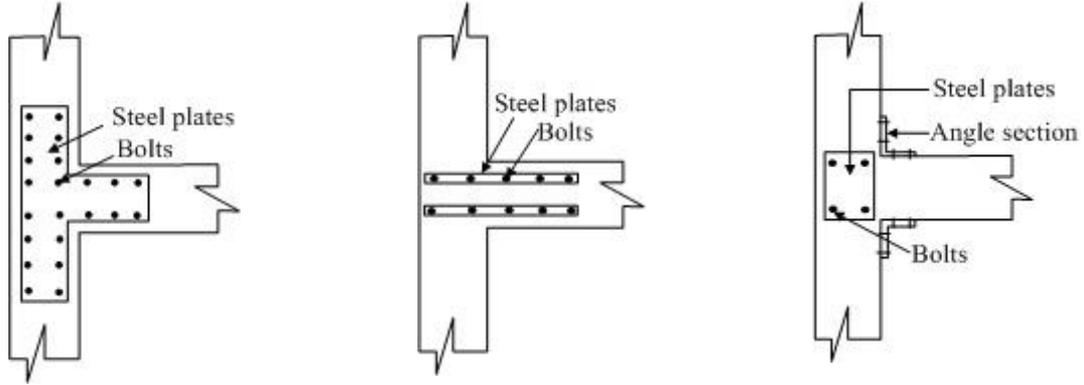
Figure 12: Strengthening of weak joints with steel plates and angle sections
