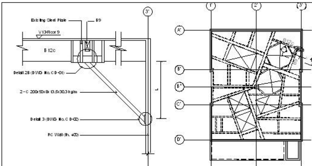
Figure 15: Strengthening of floor system by external bracing
