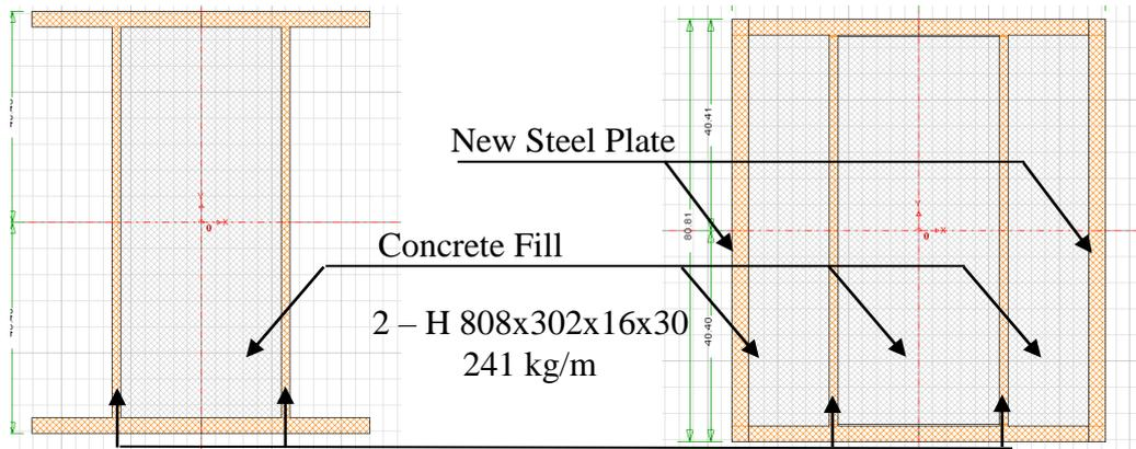
Figure 14: Strengthening Composite Column (a) Existing column (b) Column after strengthening
