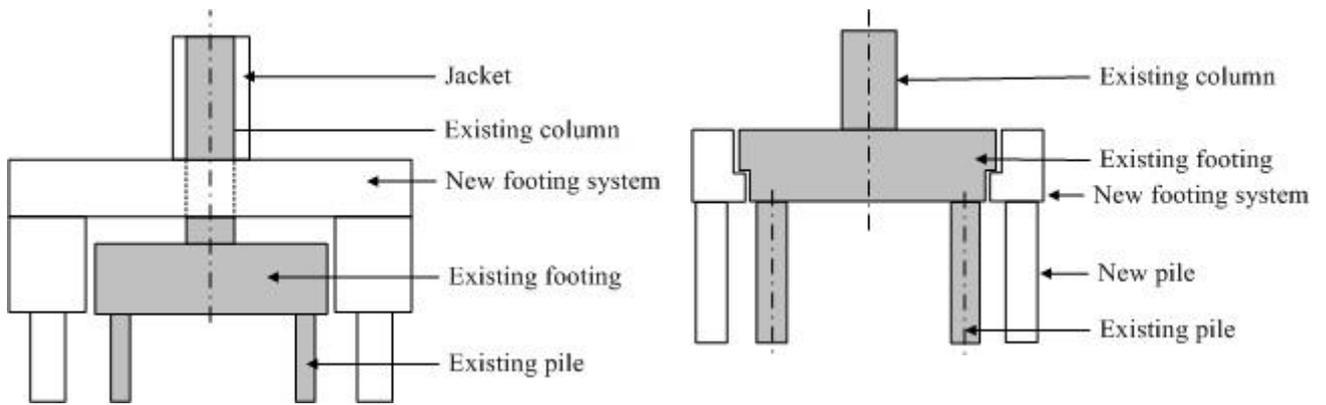
Figure 3: Strengthening of existing foundation (a) Bridging (b) Additions
