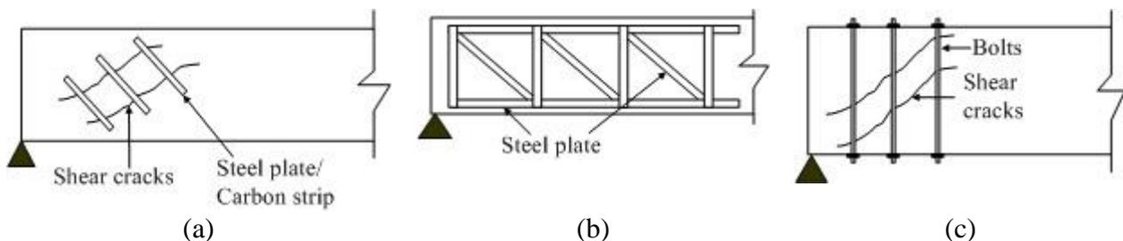
Figure 9: Strengthening of beams in shear (a) Minor deficiency (b) Major deficiency (c) Using transverse post tensioning
