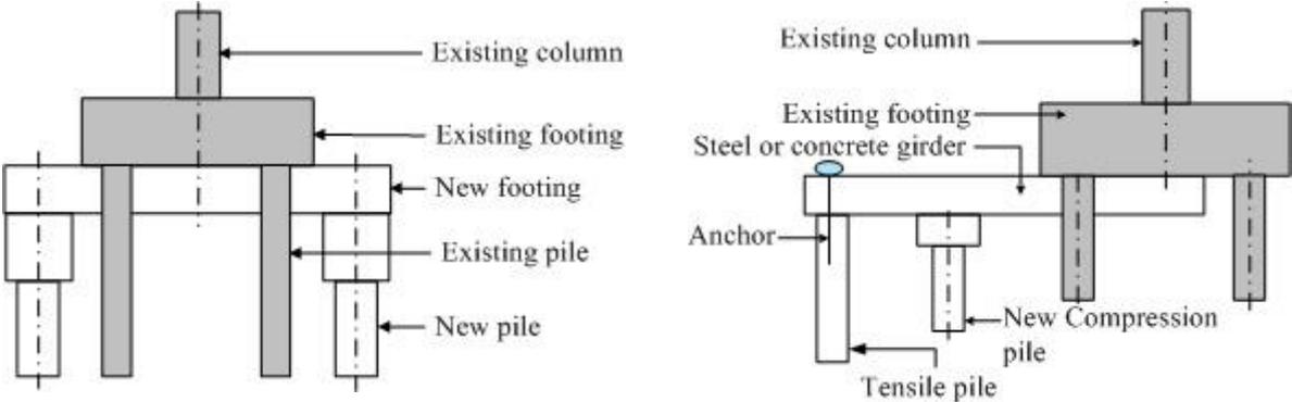
Figure 11: Strengthening of foundation by underpinning
