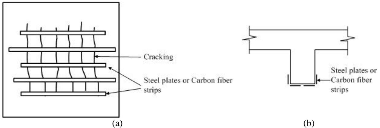
Figure 8: Strengthening of slab using steel plates and or carbon fiber strips
