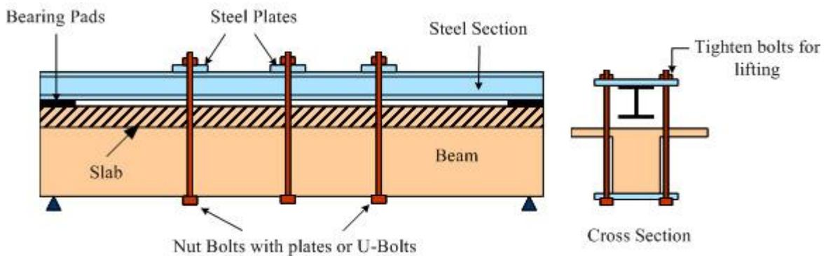
Figure 4: Overall Strengthening of beam by hanging
