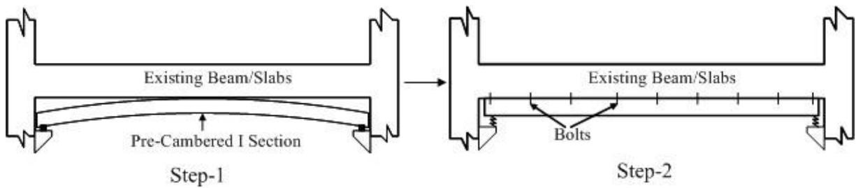
Figure 7: Jacking an excessive deflected beam by pre-cambering
