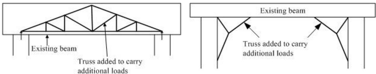
Figure 5: Strengthening by adding external truss
