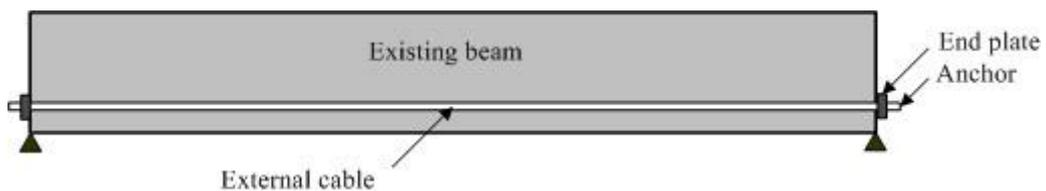
Figure 2: Post tensioning a weak beam by external cable
