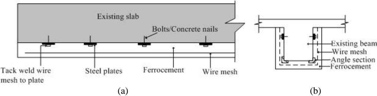
Figure 6: Strengthening of (a) slab (b) beam using steel plates and ferrocement
