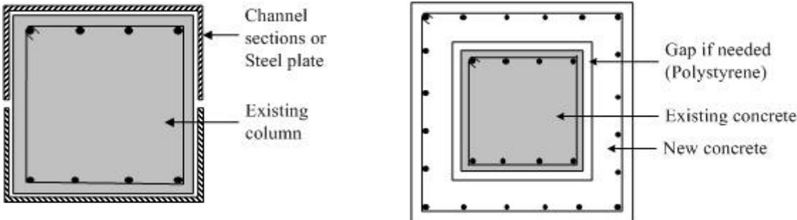
Figure 10: Strengthening of columns for axial loads
