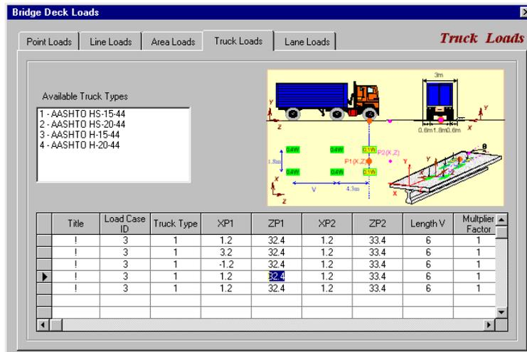
Figure 15: Modeling of the Truck Load in SAP2000
