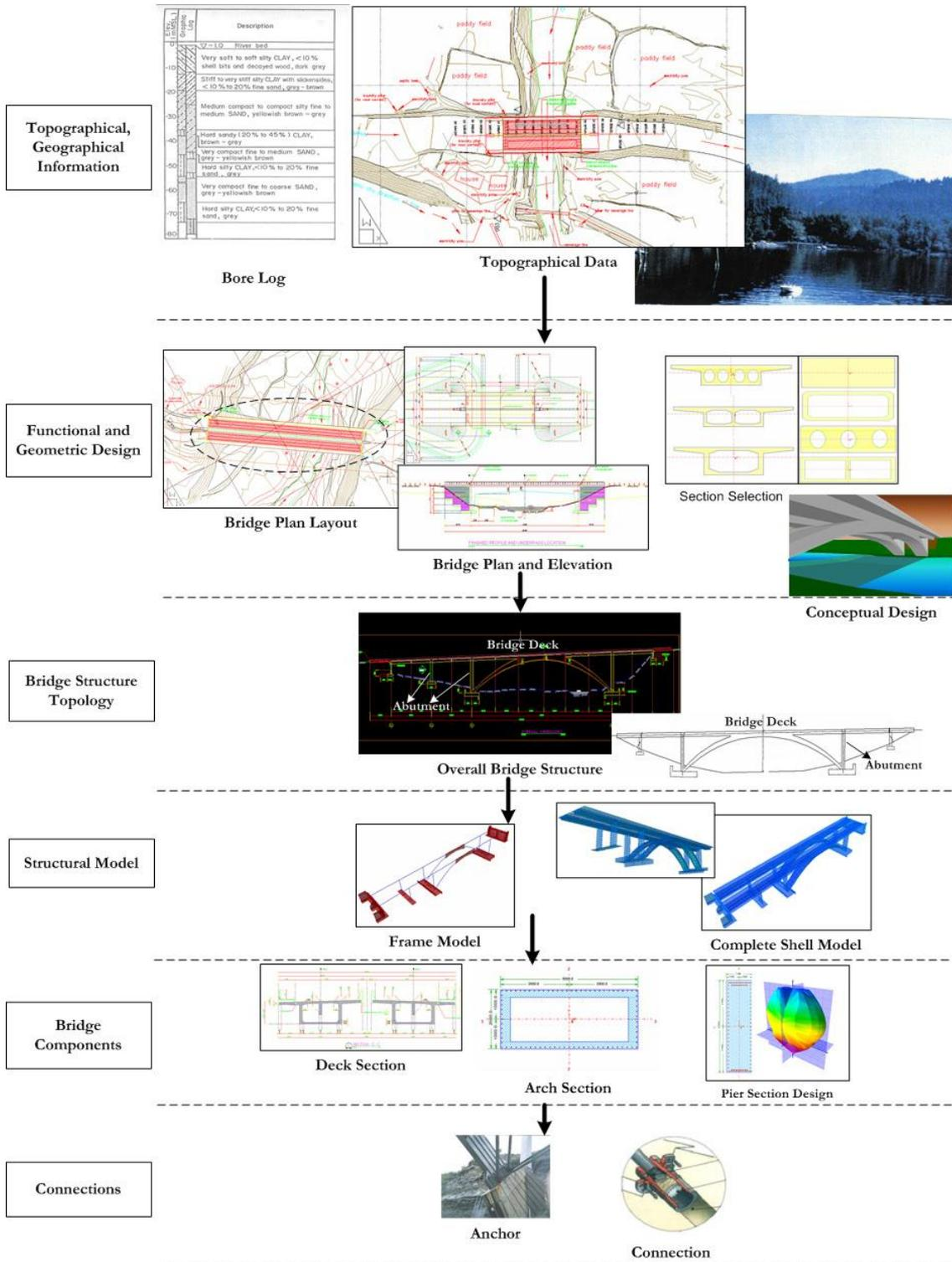
Figure 16: Hierarchical Multi-scale Design Approach for Bridge Design
