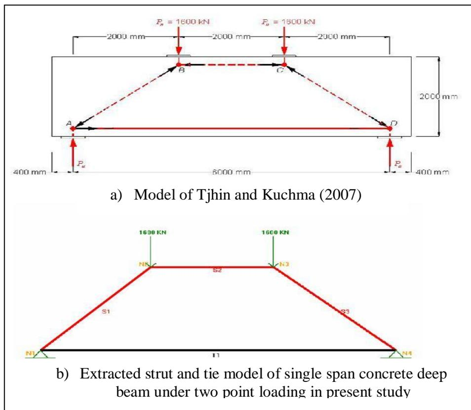
Fig 9. Comparison of extracted STM with the model of Tjhin and Kuchma (2007)
