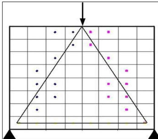
Fig 4. Linear-curve fitting for strut-and-tie lines in a single-span concrete deep beam
