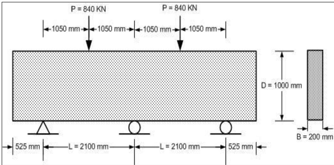
Fig 10. Two-span continuous deep beam under two point loading taken from the specimen (BM7/1.0, T1) of Rogowsky presented by Zhang and Tan (2007)
