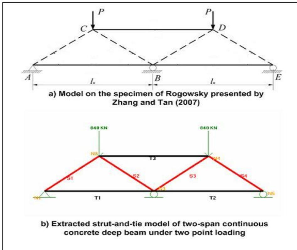
Fig 11. Comparison of models between the extracted and the existing model of the two-span continuous concrete deep beam under two point loading
