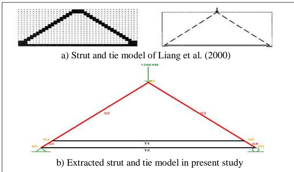
Fig 7. STM comparison for single-span concrete deep beam under single point loading
