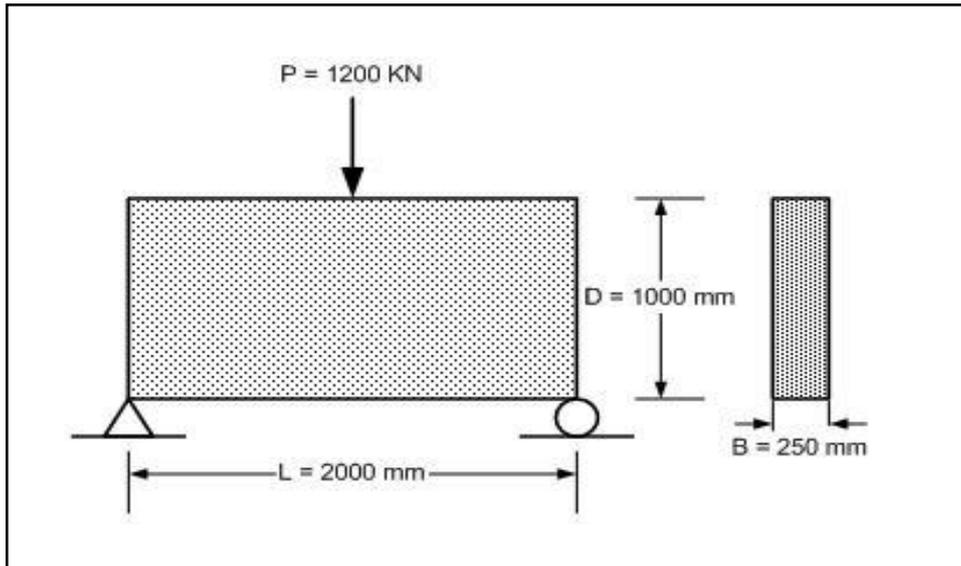
Fig6. Single-span concrete deep beam configuration under one-point loading taken from Liang et al. (2000)
