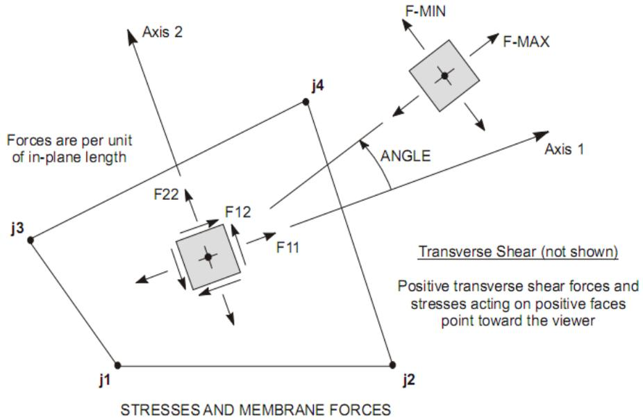
Fig 1. Shell element internal forces (SAP2000 Reference Manual)
